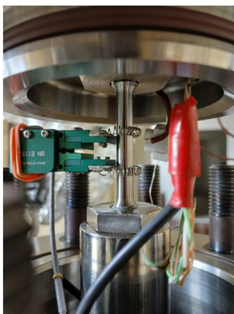
Fig. 1 Test specimen prepared for in-situ high-pressure hydrogen SSRT.
