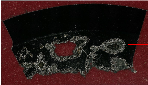
Fig. 12 Corroded area on the inner surface of the tube, graphite forms rings around holes.
