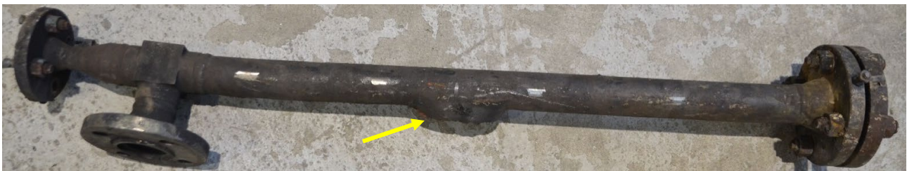
Fig. 1 Delivered tube with perforated wall.
