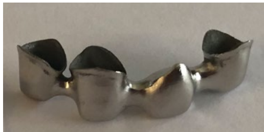
Fig. 1 Additively manufactured 3D-printed Co-Cr dental bridge.
